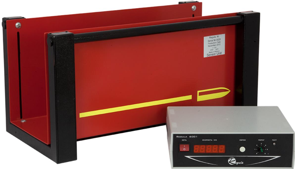
**The complex is intended for measuring bullet speed and for testing small arms and sporting/hunting weapons in the process of forensic ballistics expertise.**
